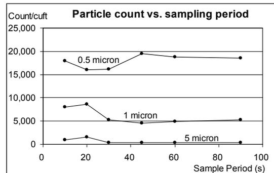
Most trials resulted in cyclic variations in downstream interval counts. It was thought this was due to periodic loading of filter media followed by periodic shedding of dust as air turbulence on media rearranged particles.
